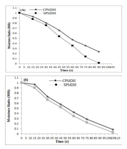
Figure 1. Moisture ratio (MR) vs. time for (A) vacuum-drying of FS-1 sample using SPMDH and CPMDH, and (B) vacuum-drying of FS-2 sample using SPMDH and CPMDH.
